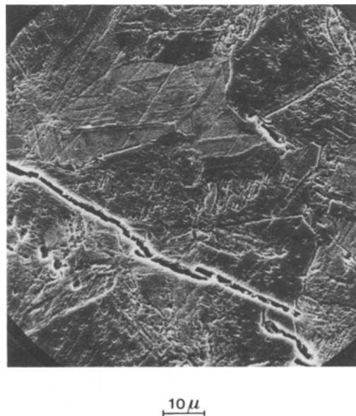
Fig. 13. Scanning electron micrograph of a section of a deposit parallel to the electrode surface.
